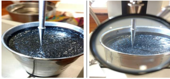
Figure 3. Softening test of enhanced polymeric bitumen.
