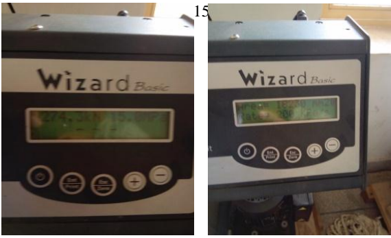
Fig.4: Setting loading rate and area of specimen
