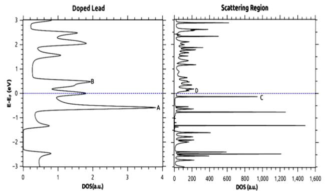
**Fig. 6.** The calculated DOS of N-doped ANGRs, and the energy levels of the isolated scattering region saturated by hydrogen atoms. When a bias voltage is applied, the relative position of narrow peaks in DOS of leads (A and B) is shifted. In the resonant tunneling regime, the junction becomes conductive when the energy position of channel state(s) in the scattering region (C and D) matches that of channel(s) in the electrodes.
