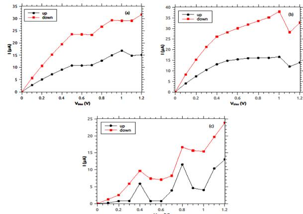
**Fig. 5.** Comparing the characteristics of the spin-dependent current-voltage ( $I-V$ ) of the (a), (b) and (c) one, two and three nitrogen doping on iron adsorbed hybrid AGNR-SiC-GNR nanoribbon, respectively (A, B and C structures)
