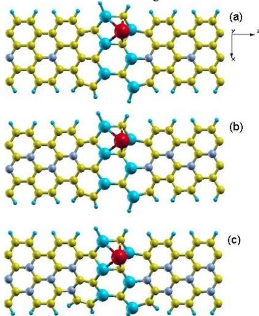
**Fig.2.** Schematic representation of the various configurations used in calculations after the relaxation of each structure. The structural symmetry is broken when a narrow Fe adsorbed armchair SiC nanoribbon is inserted between the two N-doped armchair graphene nanoribbons. (a), (b) and (c) represent one, two and three nitrogen doping on iron adsorbed hybrid AGNR-SiC-GNR nanoribbon, i.e. A, B and C structures respectively.
