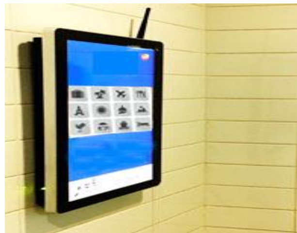
Figure (3) Digital signage supported by the antenna for remote content update purposes (Photographed at Melbourne Tullamarine airport, 2018)
