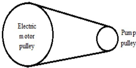
**Fig 1: 3:1 Ratio Pulley**
