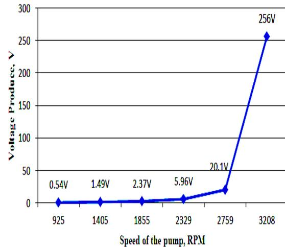
**Fig 2: Figure 2: Speed of Pump towards the Voltage Produced.**
