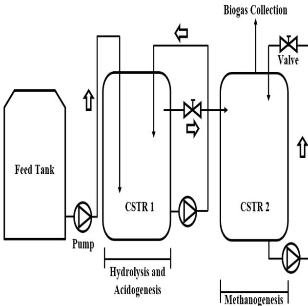
Fig. 2: Experimental Setup at Laboratory
