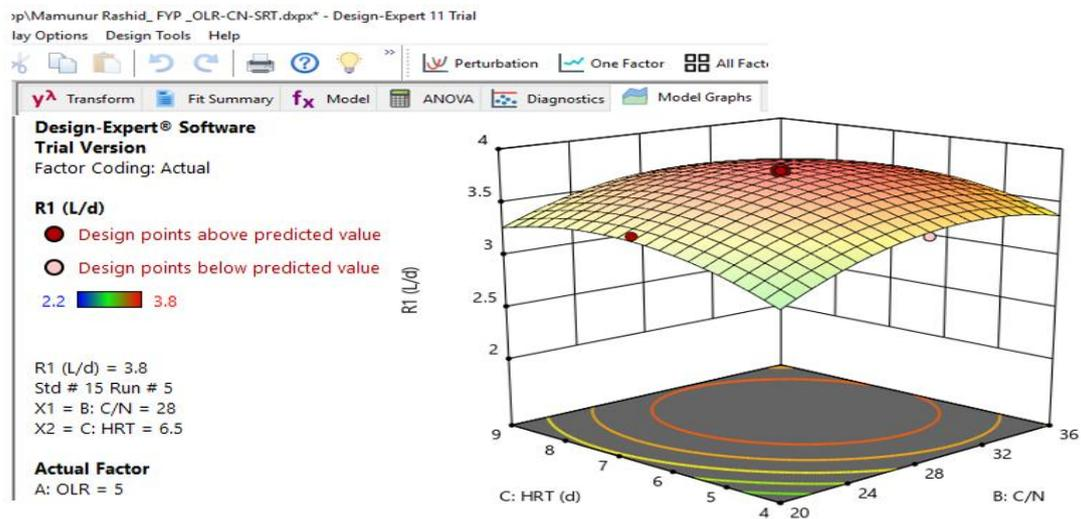
Fig. 5: Optimum Level of Biogas Production with Respect to Optimum Level of OLR and HRT as Inputs
