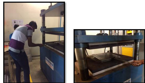
(f) This process was to heat up the fiberboard and to make it solid.
