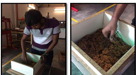
(c) The ration of the UF glue was measured perfectly and blended in a mechanical blender together with the refined fibers.
