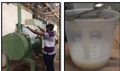
(c) The ration of the UF glue was measured perfectly and blended in a mechanical blender together with the refined fibers.
