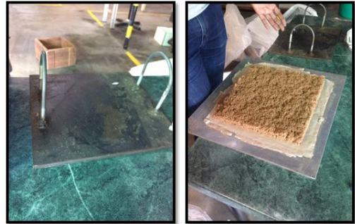
(e) A metal plate flattener was used to compress the fibers to achieve the desired thickness.
