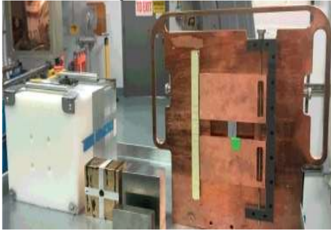
Figure 1. Defensive blocks and collimators accessible at NSRL beams. It is composed of three layers collimators which are prepared from aluminum, polyethylene, and Lucite augmented to reduce the external dosage for less than 2 percent during exposed to a 600 MeV/u 56Fe beam. It was also used for further ions for the energies that results in a related amount not more than 3%. Altered dimensions and dump arrangements are open. Brass collimators are utilized as to reduce the beam dimension and for producing comparable sketching beams. Various scopes of Tungsten chunks can achieve various collimator forms. A collimator of copper by adaptable size initially planned to shape stumpy vigorous beams.
