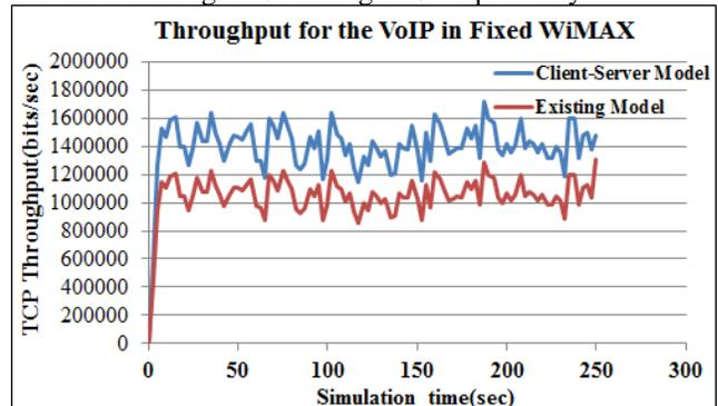
Figure 9: Scenario\_2 of the Existing and the Client-Server models throughput for VoIP Results
