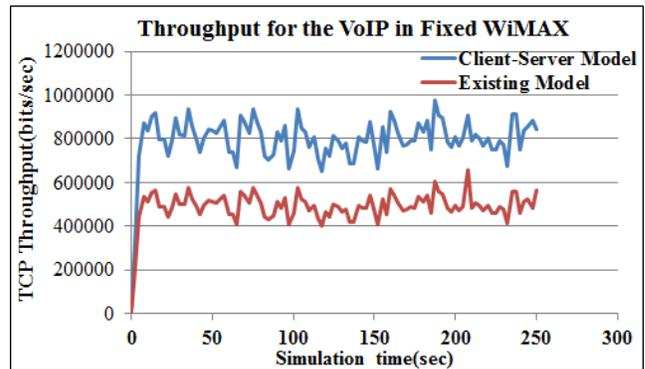
Figure 8: Scenario\_1 of the Existing and the Client-Server models throughput for VoIP Results
