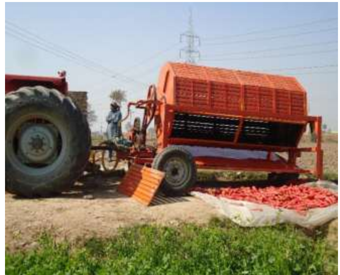
Fig. 5: Tractor Operated Carrot Washer
