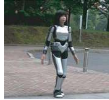
Figure 3 HRP-4C Humanoid: stable walking under linear inverted pendulum model [4]
