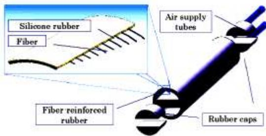
Fig (1) A two chamber pneumatic soft actuator [18].
