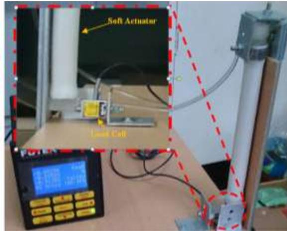
**Fig(4) Bending Force measurement**
