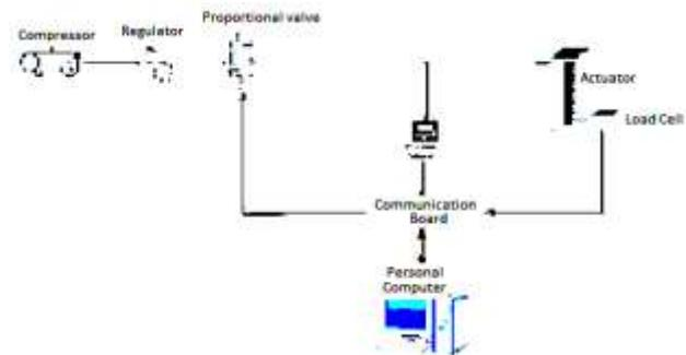
Fig (2) Hardware schematic diagram for the System Identification process
