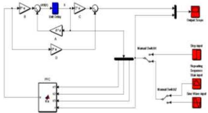
**Fig 5(b) Simulink Block Diagram of Model interfaced with PFC Controller**
