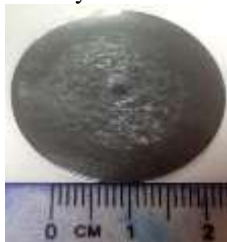
Fig (2) A disk shaped sample was prepared for Ti-6Al-4V and SUS 316L with 0.7 mm thickness.
