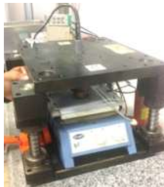
Fig (3) Interfacial contact resistance (ICR) apparatus.
