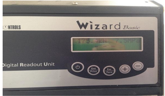
Fig. 12. Load Applied in KN and Compressive strength in MPa.
