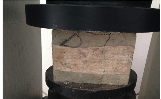
Fig. 11. Crack appeared on the surface of cube.
