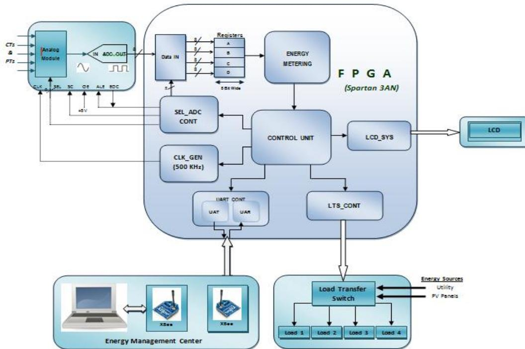
Fig.2. Hardware Architecture of Smart Energy Management System
