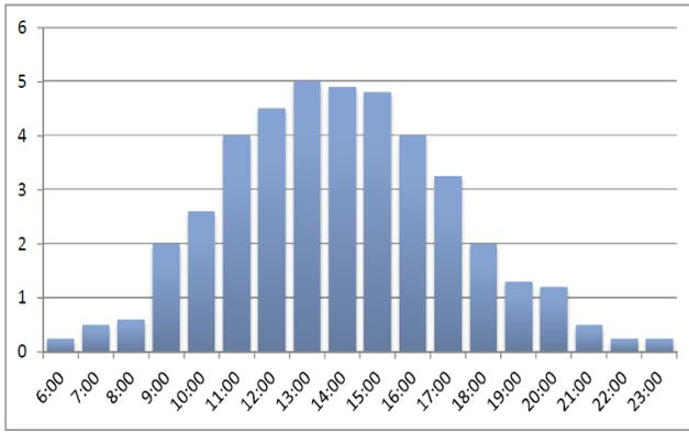
**Fig.10. Hourly variations of power consumption w.r.t time in normal load control technique**
