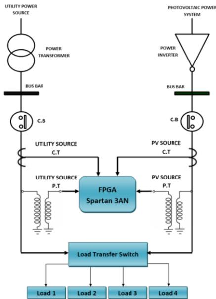
Fig.4. Single Line Diagram of SEMS
