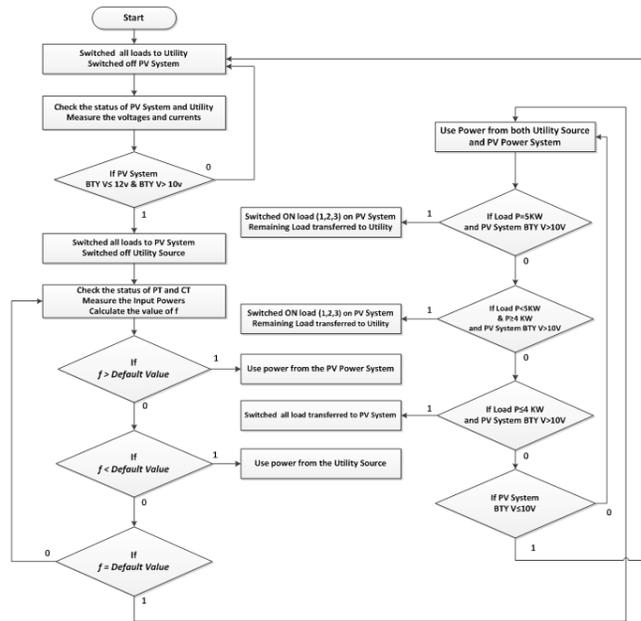
Fig.6. Algorithm of Efficiency Based Technique.
