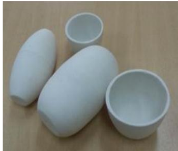
Fig (1) Examples of hollow porcelain products produced via CRSM (Adapted from [6])
