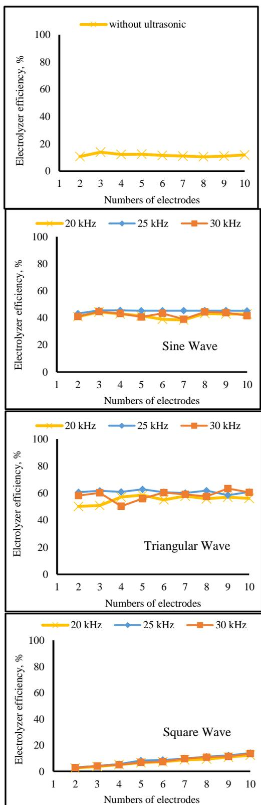
Figure 10 Electrolyzer efficiency under the different treatments
