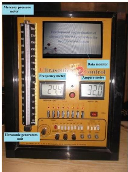
Figure 1. Ultrasonic-Hydrogen Electrolyzer System (UHES)
