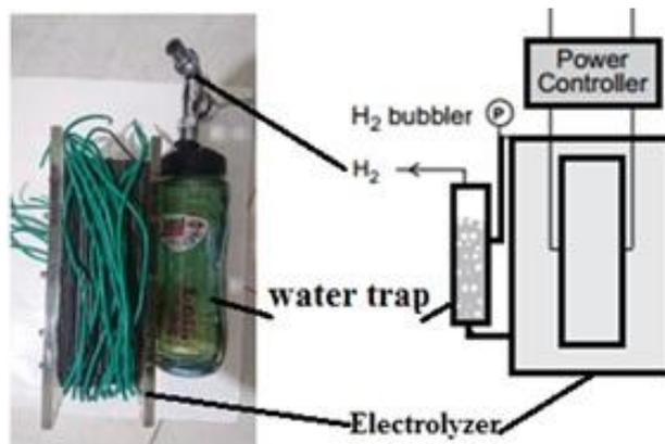
Figure 3. Bubblers (water trap).
