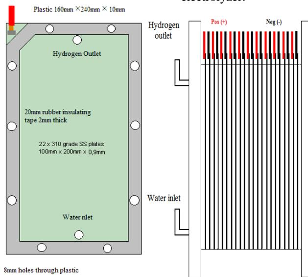
Figure 2. The water electrolyzer
