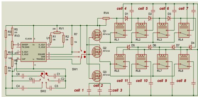
Figure 5. The schematic circuit diagram of ultrasonic Power Amplifier
