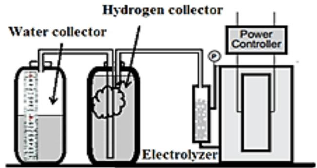
Figure 6 The water displacement system.
