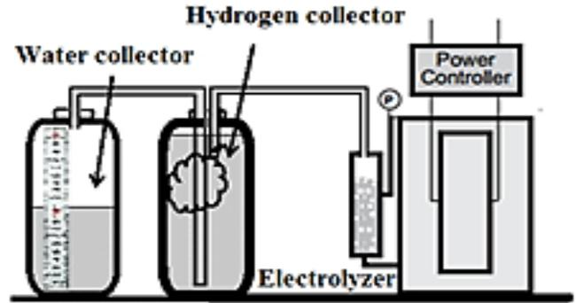
Figure 6 The water displacement system.
