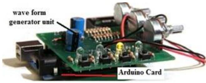
Figure 4 Arduino waveform Generator.
