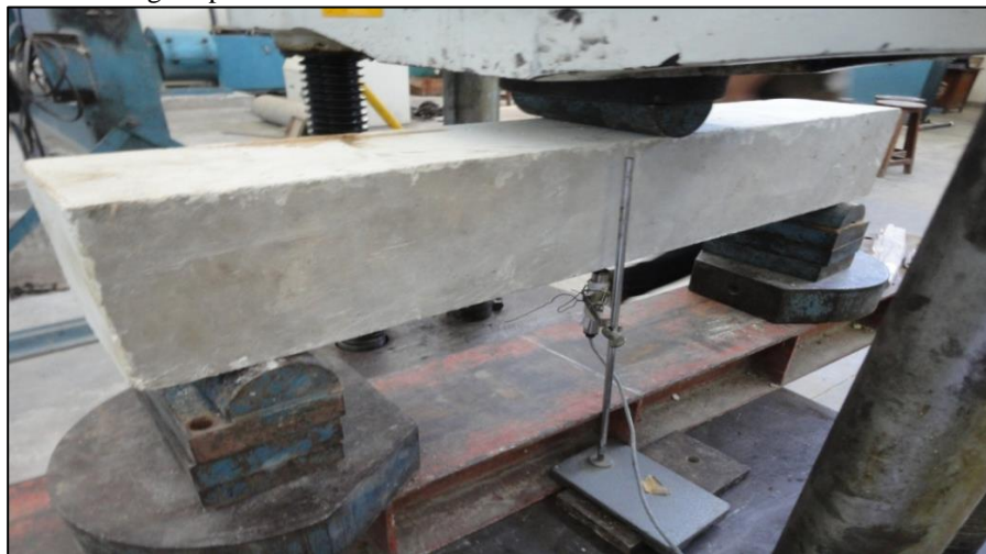
Figure.1 Computerized UTM for determination of load carrying capacity of RCC beams
