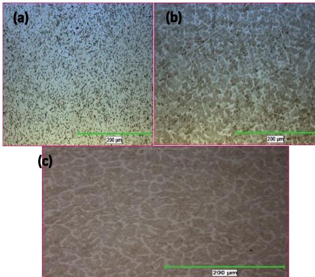
Fig 1. The surface micrographs of the hardfacing alloys: (a) Alloy-1 (b) Alloy-2 (c) Alloy-3
