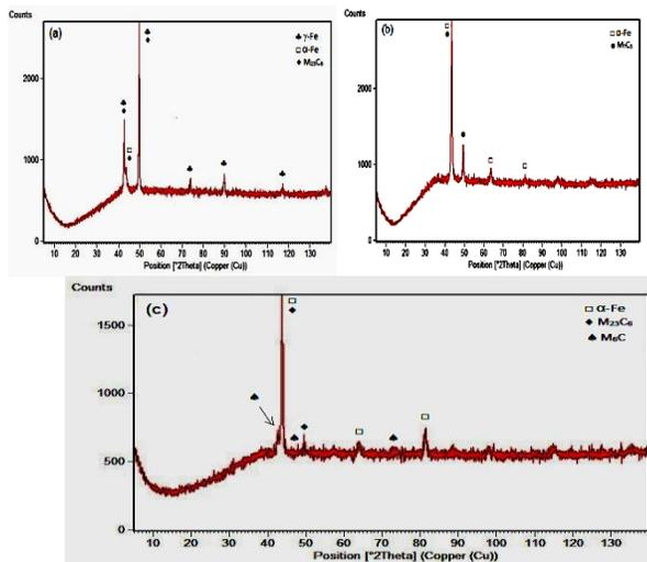
Fig. 2. XRD patterns for the different conditions: (a) Alloy-1 (b) Alloy-2 (c) Alloy-3
