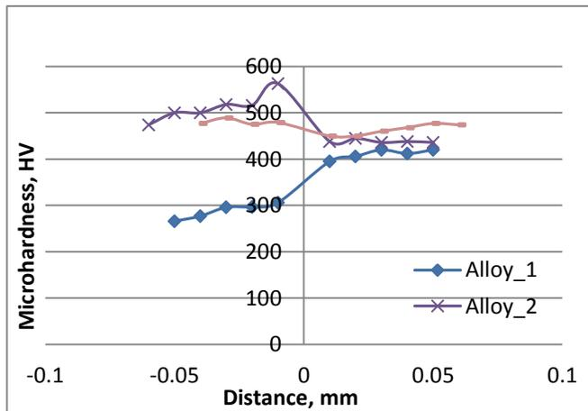
**Fig. 4. The hardness curve of the hardfacing depth profile**
