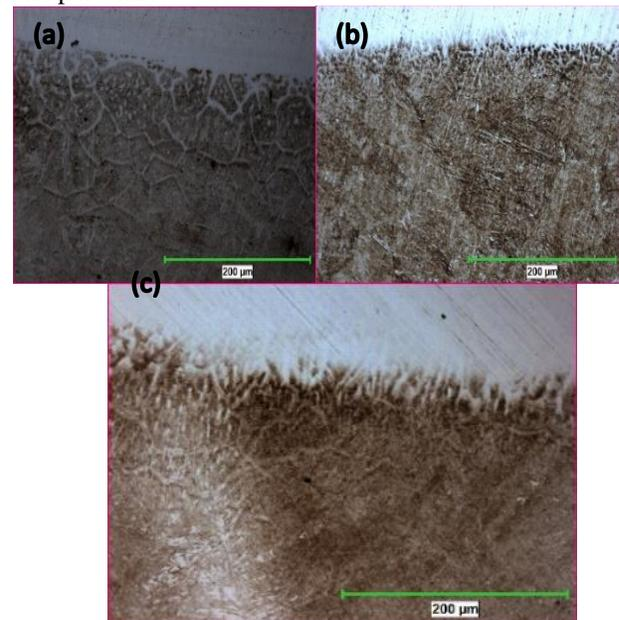
Fig.3. SEM of the hardfacing layers (a) Alloy-1 (b) Alloy-2 (c) Alloy-3
