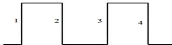
Fig. 2 Double barrier structure, the numbers identify the interfaces
