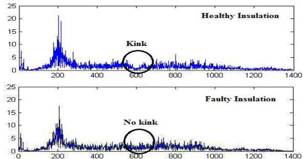
Fig. 12 Comparison between FFT plots for healthy and faulty insulation condition (Internal discharge)
