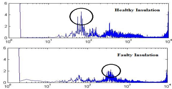
Fig. 11 Comparison between FFT plots for healthy and faulty insulation condition (External discharge)
