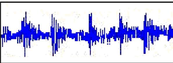
Fig. 15 Signature of external discharges
