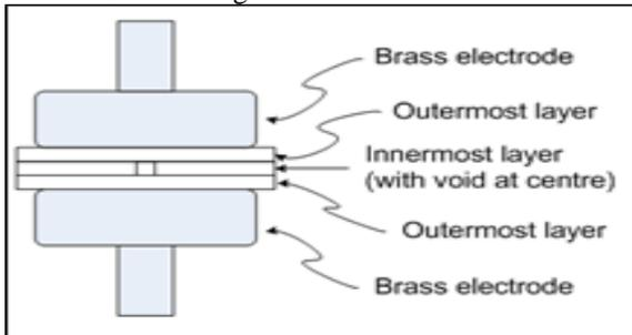
Fig.4 Creation of internal discharges.
