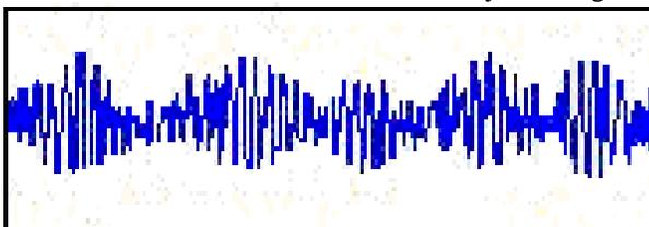
Fig. 16 Signature of internal discharges
