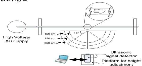
Fig.1 Equipment setup for external discharges.
