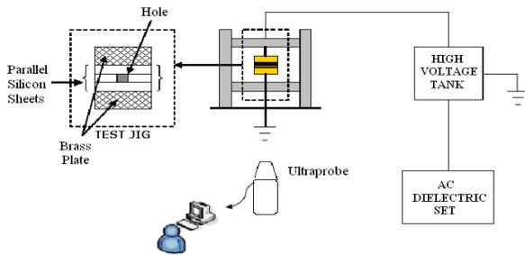
Fig.2 Equipment setup for internal discharges.
