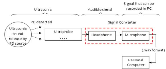
Fig.5 Block diagram of Signal Converter System.
