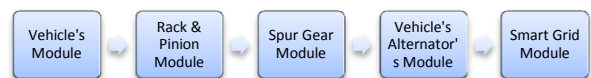
Fig. 2. Block Diagram of Vehicles Kinetic Energy Converter Reported to an actual status of Pakistan, there is an immense traffic magnitude on wayside. The transports necessarily travel over the bumps when an individual
