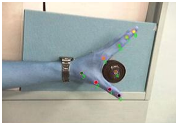
Figure (5) Image processing based marker less motion capture analysis using calibrated stereo camera to determine range of motion normal fingers.
