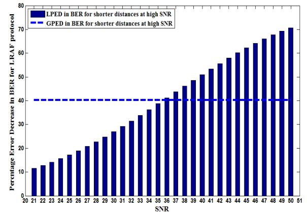
Fig .10. The PED comparison with PPAF three time slots protocol for shorter distances and medium to high SNR values
