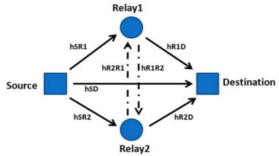
**Fig. 1. Inter-relay communication using LRAF TDMA- based three times slots protocol**
