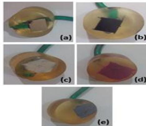
**Fig. 1 Snapshot of (a) Bare sample (boiler tube), (b) Paint-primer sample, (c) Painted Sample, (d) Primer sample, (e) Ni-Cr coated**
