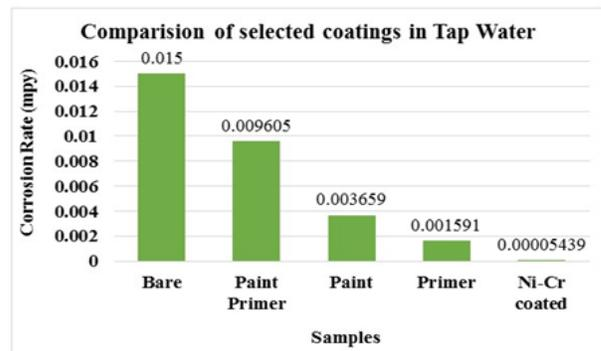
Fig. 3 Comparison between coated Samples
