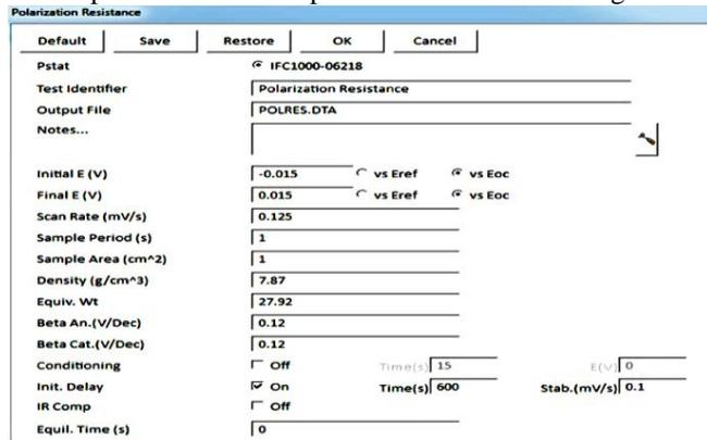
Fig. 2 Snapshot of parameters used in LPR test
