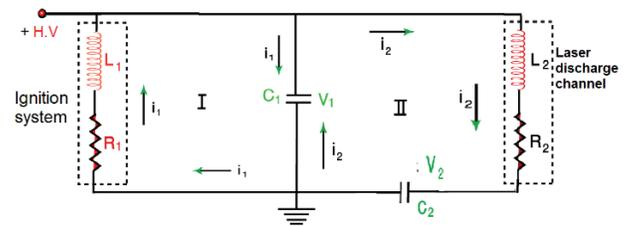
Figure (b). Equivalent Blumlein circuit
