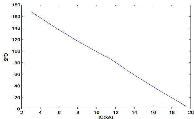
Figure 8. SFO for simulated system without shield wire.
