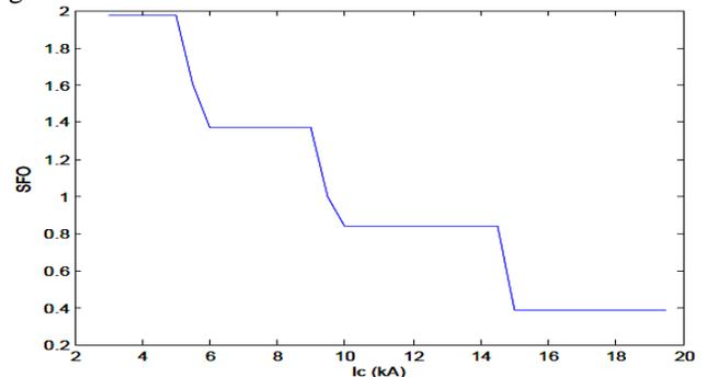
Figure 7. SFO for simulated system (shielding angle =  $57^\circ$ , one shield wire)
