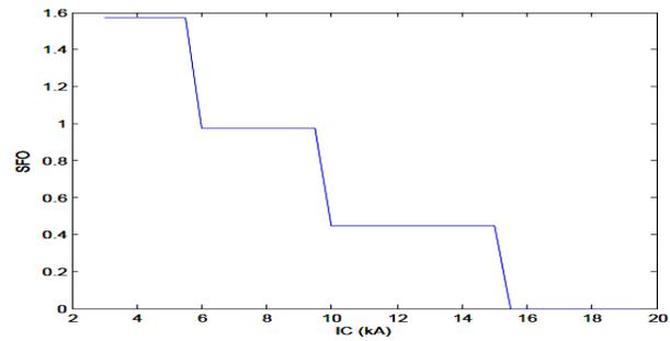
Figure 5. SFO for simulated system (shielding angle =  $60.36^\circ$ , computed by EGM).
