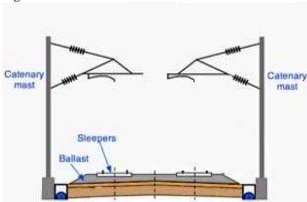
Figure 2. Electric railway overhead feeding system.
