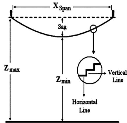
Figure 3. Shielding and feeding wires modeling.
