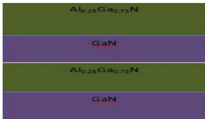
Fig. 1: Nitride double barrier heterostructure showing composition of layers
