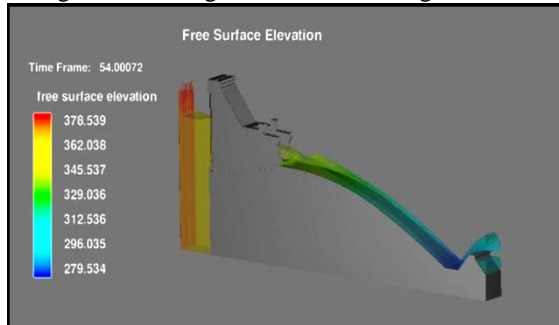
Figure 4: Flow Simulation at 10.67 m Gate Opening
