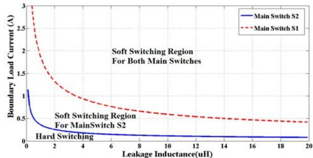
Figure 7. Soft switching operation.
