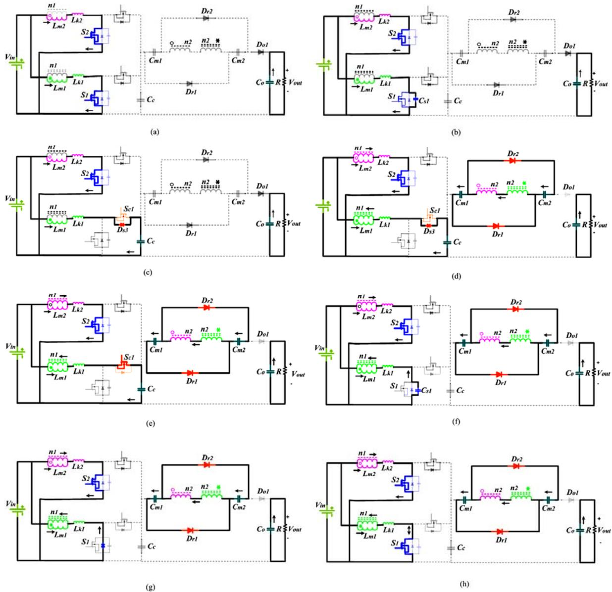
Figure 4. Operation processes of proposed converter: (a) Stage 1 [t<sub>0</sub>-t<sub>1</sub>]; (b) Stage 2 [t<sub>1</sub>-t<sub>2</sub>]; (c) Stage 3 [t<sub>2</sub>-t<sub>3</sub>]; (d) Stage 4 [t<sub>3</sub>-t<sub>4</sub>]; (e) Stage 5 [t<sub>4</sub>-t<sub>5</sub>]; (f) Stage 6 [t<sub>5</sub>-t<sub>6</sub>]; (g) Stage 7 [t<sub>6</sub>-t<sub>7</sub>]; (h) Stage 8 [t<sub>7</sub>-t<sub>8</sub>]
