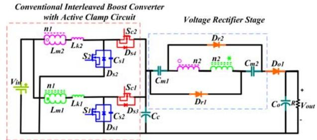
Figure. 1. Proposed non-isolated ZVT boost converter with coupled inductors and switched capacitor.
