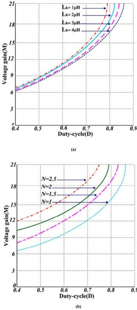
Figure 5. Voltage gain of proposed converter: (a) voltage gain with different leakage inductances; (b) voltage gain with different turns ratio.
