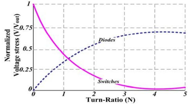
Figure 6. Relationship between normalized diodes and switches voltage stress with turns ratio.
