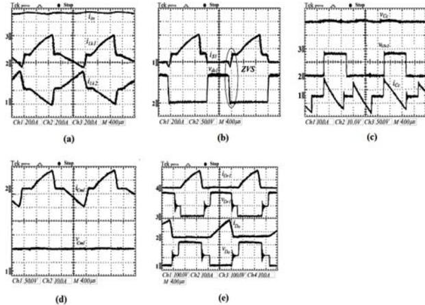
Figure 8. Fig.8 (a) to Fig.8 (e) show the waveform of the proposed converter at full load state with 30V input voltage.
