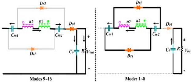
Figure. 3. The current flow-path in the voltage rectifier stage in the whole switching period.
