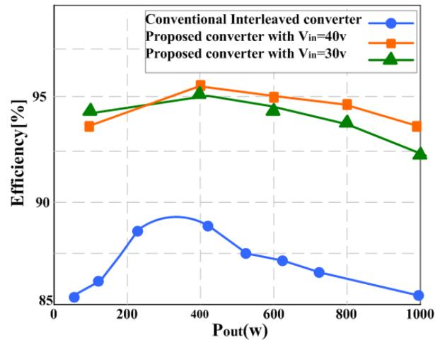
Figure 9. The efficiency comparison with the investigated topology and the conventional interleaved converter at various loads with different input voltages.
