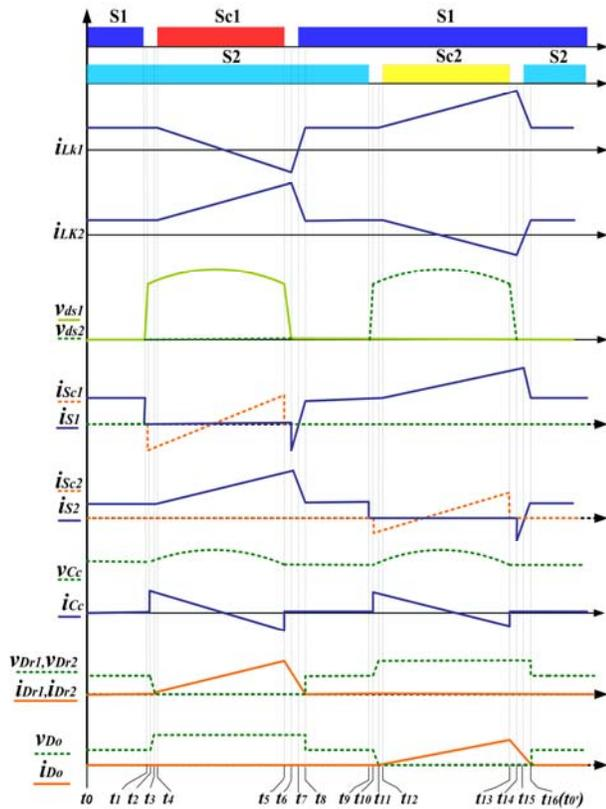
Figure 2. The theoretical waveforms of the proposed converter.
