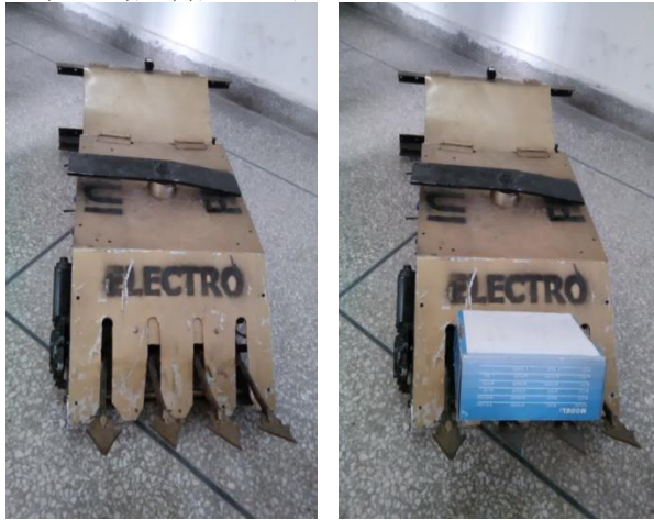
(a) (b) Figure 3 No load and carrying load on UGV
