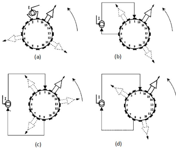
**Figure 2. Current drives for single current source EIT systems (a) adjacent (b) cross (c) polar (d) pseudo-polar [7]**
