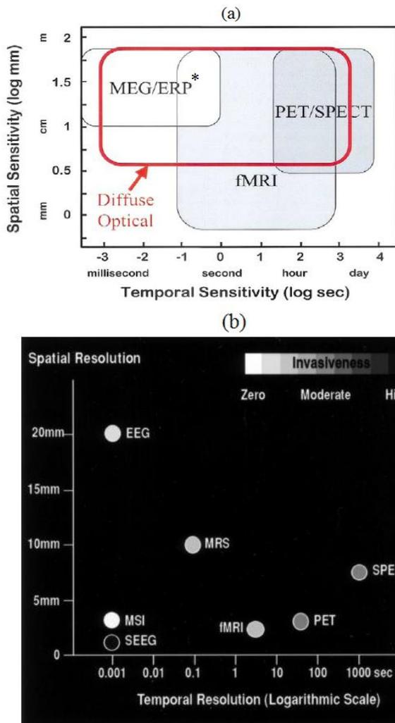
Figure 3. Comparisons of spatial and temporal resolutions of different neuroimaging techniques (a) [43] (b) [42]
