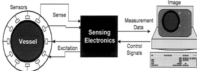
Figure 1. An electrical tomography system [1]
