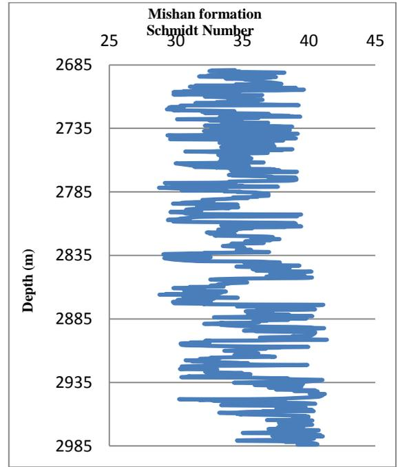
Figure 4. Schmidt rebound number for Mishan formation – Continuous estimation of UCS value of the well length (as in Figure 5 and 6)
