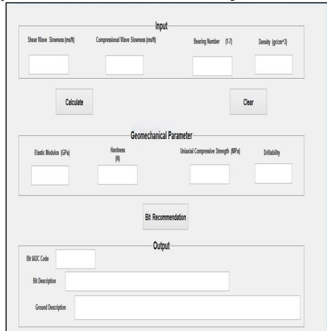
Figure 7. Software Graphical User Interface for interactive bit selection
