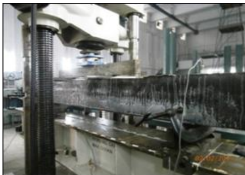
Fig.4: Two point flexure loading test setup
