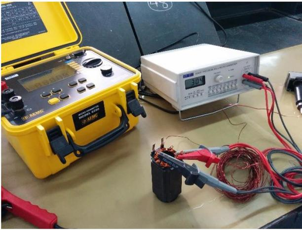
Figure 4: Resistance measurement using micro-ohmmeter
