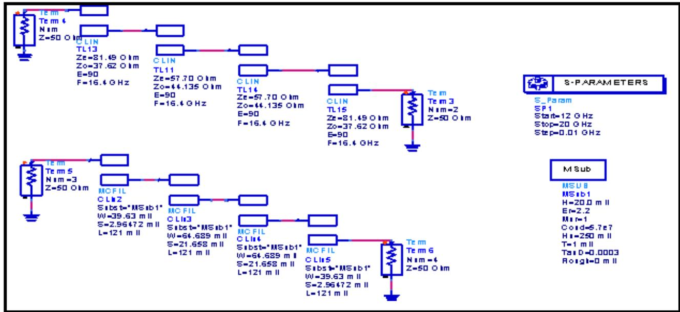
Figure 2. Ideal Transmission lines and Microstrip Transmission lines Filters on ADS
