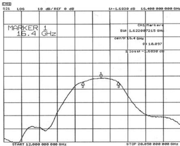
**Figure 9. Response of physically implemented Symmetric Coupled Line Band Pass Filter**
