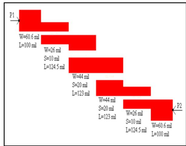
Figure 6. Momentum Layout on ADS for physically implemented filter
