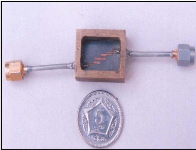
**Figure 8. Photograph of implemented Symmetric Coupled Line Band Pass Filter**
