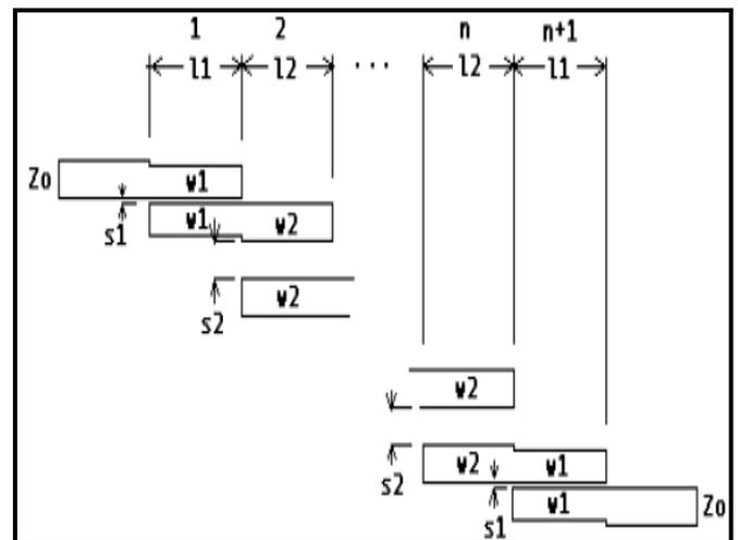
**Figure 1. Symmetric coupled line band pass filter**
