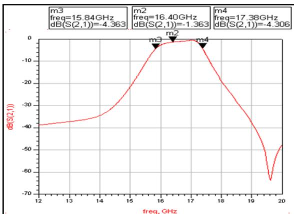
Figure 5. Full wave analysis result of optimum filter
