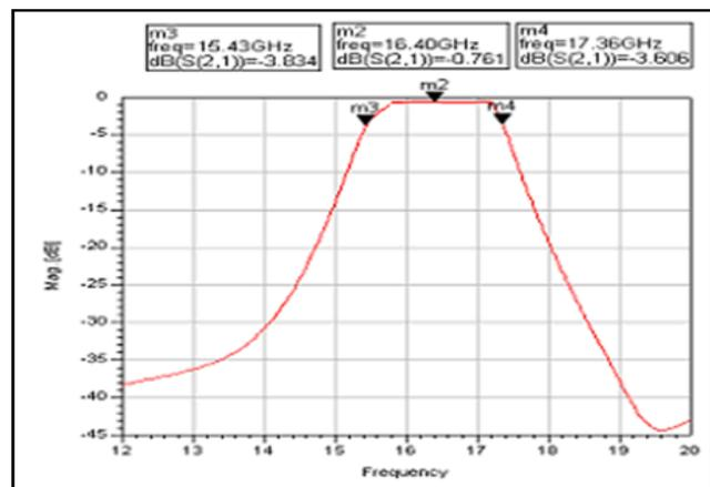
Figure 7. Full Wave Analysis of physically implemented filter
