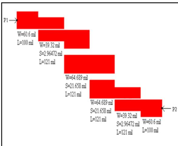
Figure 4. Momentum Layout on ADS for the optimized filter
