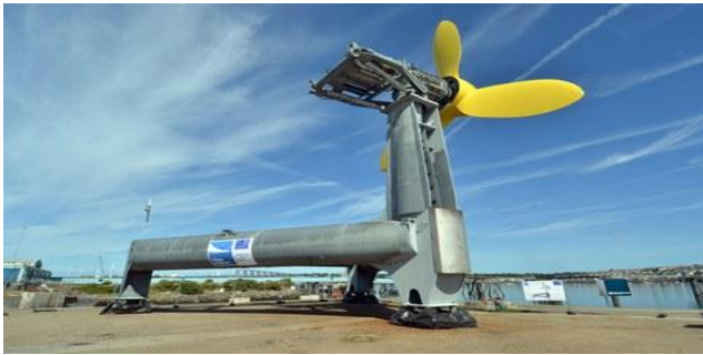
Figure 8b : 400kW Delta Stream model at Pembroke Port [35] Ocean Flow Energy Ltd
