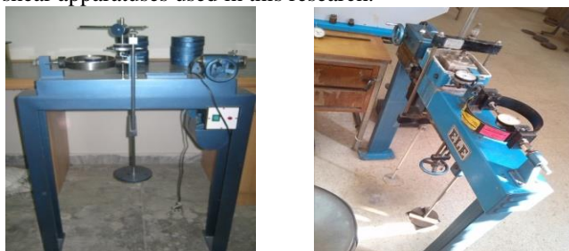
Figure3: Direct shear test apparatus a) Circular shear box b) Square shear box
