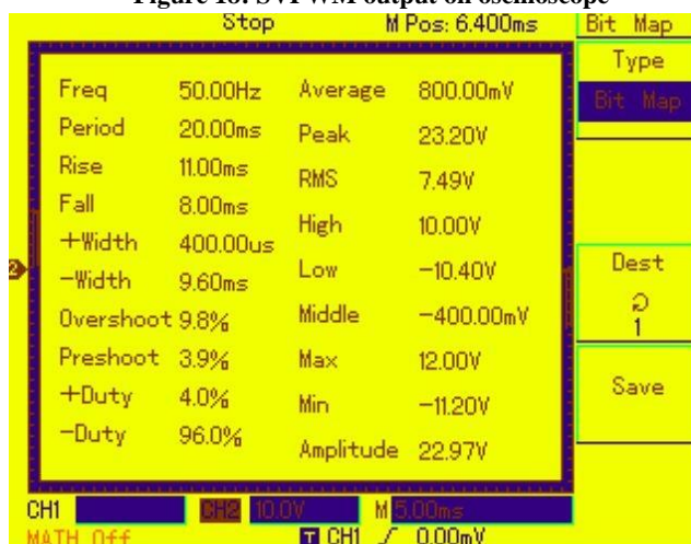
Figure 19: SVPWM parameters on oscilloscope
