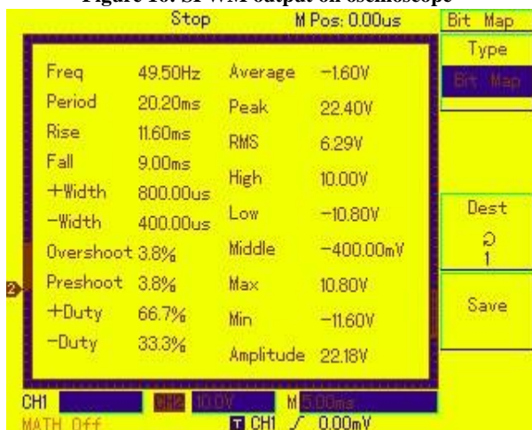
Figure 17: SPWM parameters on oscilloscope
