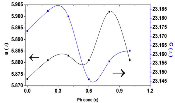
Figure 3.3: Variations in lattice parameters as a function of Pb conc(x)
