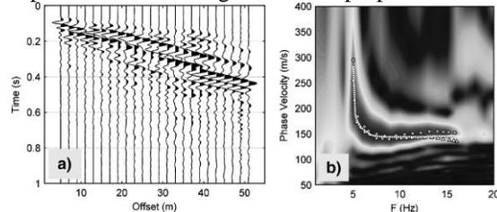
Figure 9 : Illustration of MASW data and dispersion curve(130).
