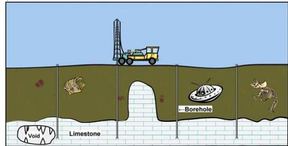
Figure 8: Conventional drilling and limestone pinnacle (Anderson et al., 2008).
