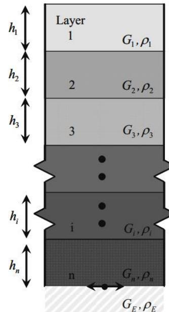
Figure 15: Model for soil column with shear modulus ( $G$ ) and density ( $\rho$ ) at horizontally layered soil deposit.
