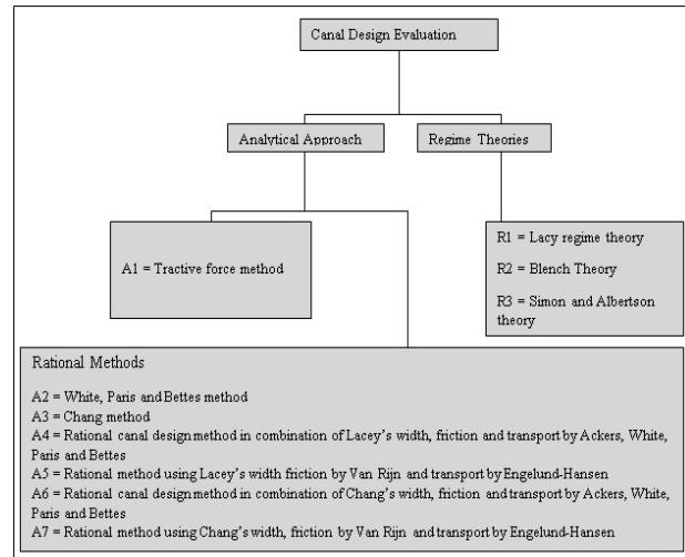
**Figure 2. Canal design evaluation framework**
