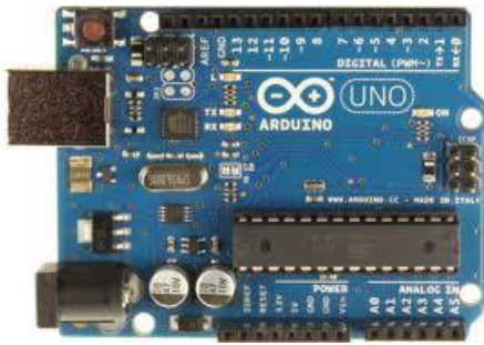
Fig. 1 Arduino UNO Board having Atmega328 Microcontroller
