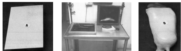
Fig: 2 Orthosis fabrication process through vacuum forming
