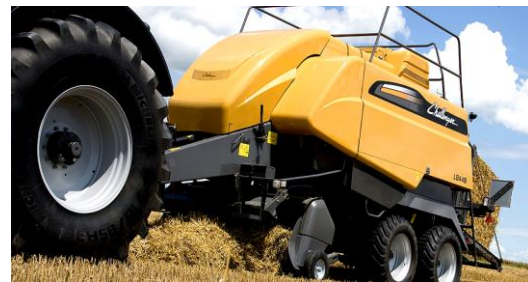
Figure 1.5. Ready bales coming out from the rear end of big baler machine.
