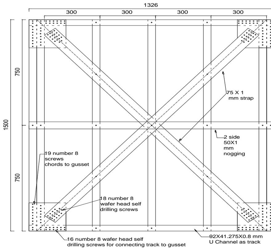
Figure 1. Prototype LSF braced frame
