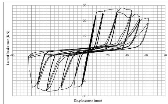
Figure 4. hysteresis behavior of LSF frame specimens
