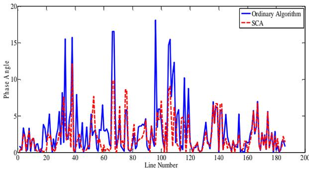
Figure 5 Comparison among compensated phase angles of ordinary algorithm and SCA
