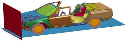
**Figure 4 FE model of the child dummy restrained in CRS for frontal crash test**
