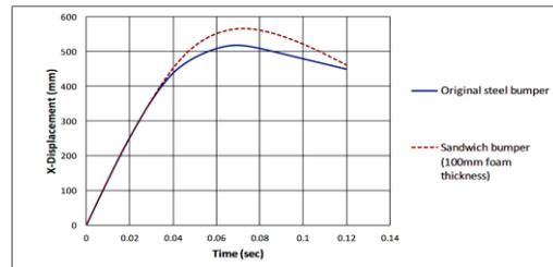
**Figure 7 Deflection-time graphs of sandwich and steel bumper**
