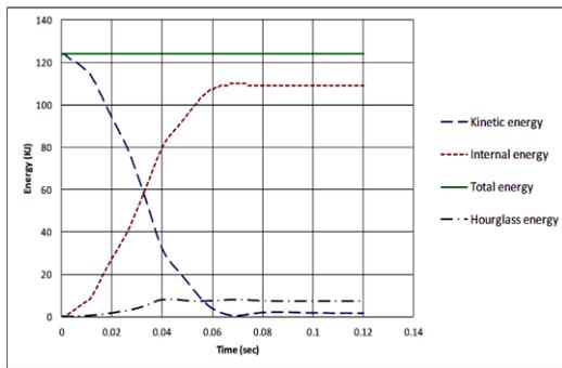
**Figure 5 Energy balance of crash with original steel bumper**
