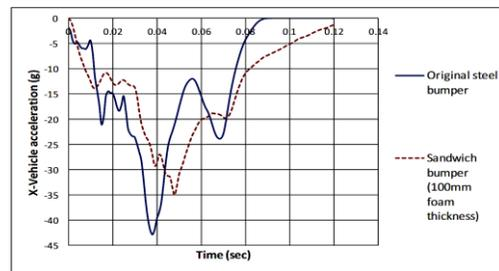
**Figure 8 Vehicle deceleration comparisons for sandwich and steel bumper**
