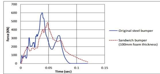
**Figure 6 Crush force-time graph of steel and sandwich bumper**
