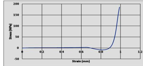
**Figure 2 Engineering stress-strain curve of the low density foam used for sandwich bumper**
