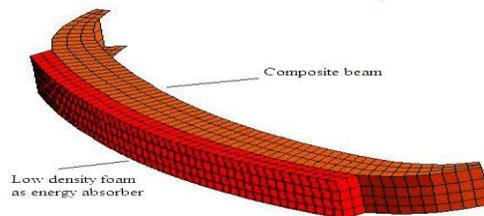
**Figure 3 Sandwich bumper beam**
