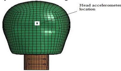
**Figure 1 Accelerometer location in the 3YO child dummy FE model head**
