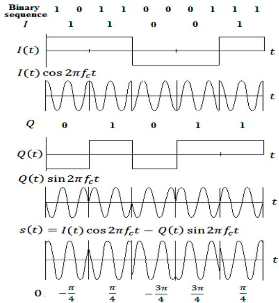
Figure 03: Theoretical wave form of QPSK Modulator
