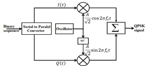
Figure 02: Block Diagram of a QPSK Modulator [5]
