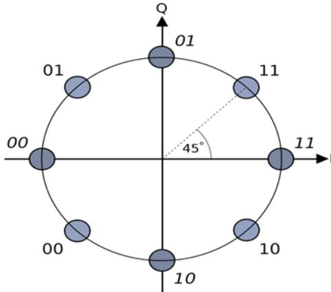
Figure 01: Constellation Diagram of QPSK [5]
