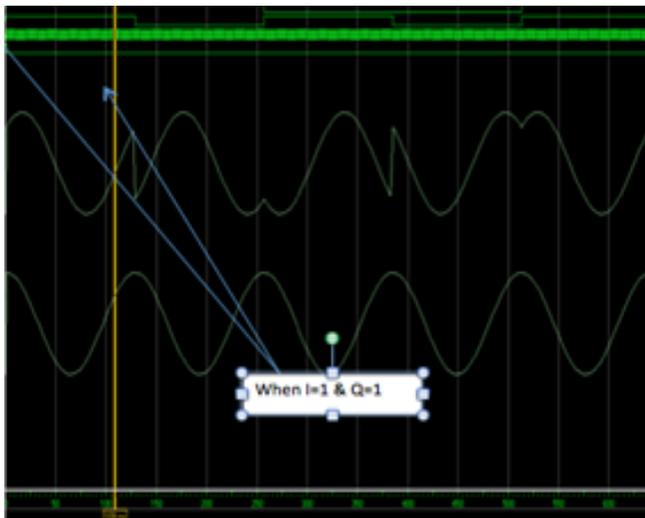
Figure 04: Justification of QPSK Modulator with (I) and (Q) bit streams.
