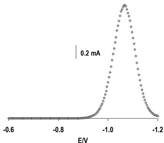
**Fig. 2: Simulated differential pulse voltammogram for the cathodic scan of 0.7 mM 2-[3,5-bis(1,1-dimethylethyl)-4-oxo-2,5-cyclohexadien-1-ylidene]acetonitrile; parameters as per established schemes [5] based on approximate explicit equations in differential pulse voltammetry**
