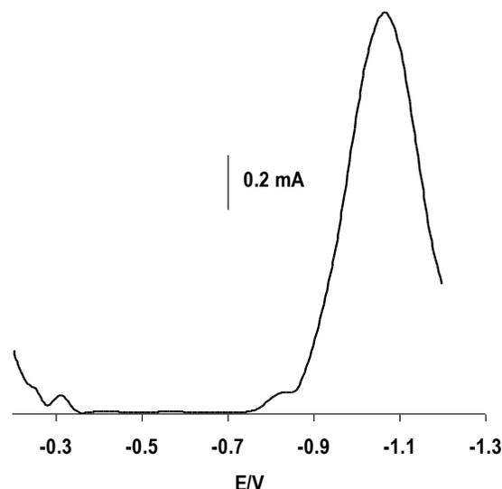
**Fig. 1: Cathodic differential pulse voltammogram of 0.7 mM 2-[3,5-bis(1,1-dimethylethyl)-4-oxo-2,5-cyclohexadien-1-ylidene]acetonitrile at platinum in 0.1 M sodium perchlorate in acetonitrile solution**
